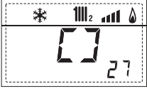
28. Visualisation valve opening control with board ZONA MIX 2 (respectively ON and OFF)
